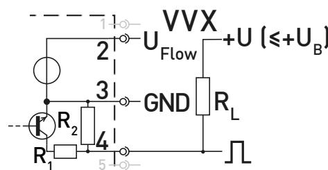
$R_1 < 47 \Omega / R_2 > 10 \text{ k}\Omega$
